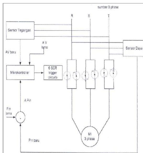
Gambar 6. Blok Diagram SCR Motor Controller
